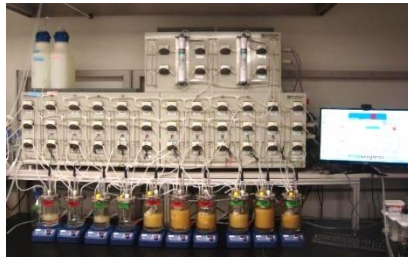
BabySHIME (Simulator of the Human Intestinal Microbial Ecosystem) (PERITOX)
